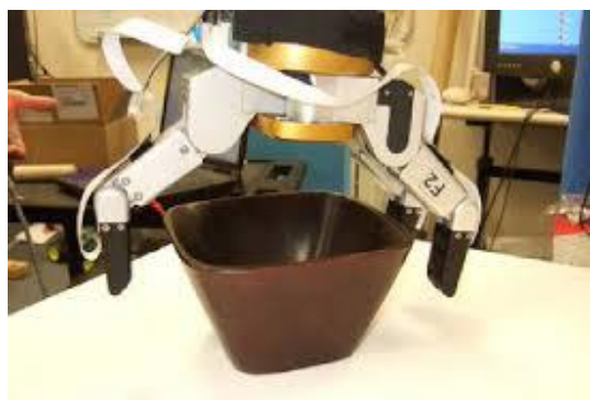
Fig6: Three-fingered Barrett Hand with our optical proximity sensors mounted on the finger tips[5].
